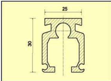
Material: AlMgSi 0.5 Heat treated anodized aluminum
