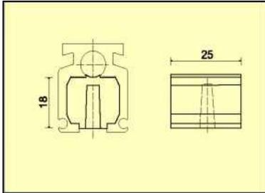
Its function is to close the ends of the curtain tracks. It is made of soft cast VULKOLLAN, and can be rigged using the threaded pin.
