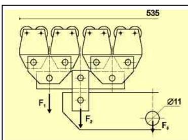
Max. load :  $F_1=30$  kg  $F_2=60$  kg  $F_3=120$  kg
