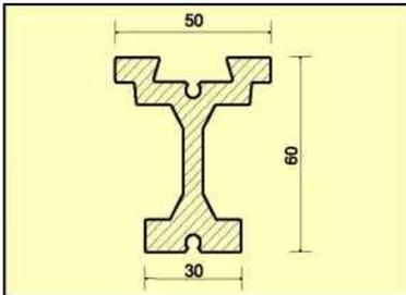
Material: AlMgSi 0.5      Heat treated anodized aluminum
