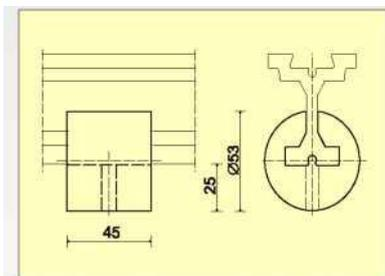
Its function is to close the ends of the curtain tracks. It is made of soft cast VULKOLLAN. It can be rigged using the threaded pin.
